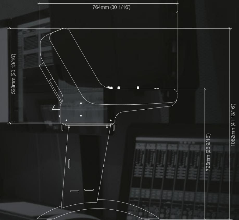
S400 is a fixed layout control surface that is available in 16+1, 32+1 and 48+1 fader configurations.
